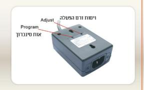
Projector AC trigger is a kind of intelligent radio transmitter, work with projector and projection screen. When projector power on, projector AC trigger detects AC power input, and will send message to projection screen, then projection screen will run down automatically; When projector closed, projector AC trigger detects no power, and will send  $message \ to \ project \ screen \ let \ projection \ screen \ draw \ back \ automatically,$ realize unmanned operation.
